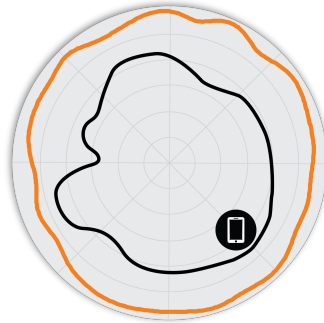
Figure 3. R650 5GHz Azimuth Antenna Patterns
